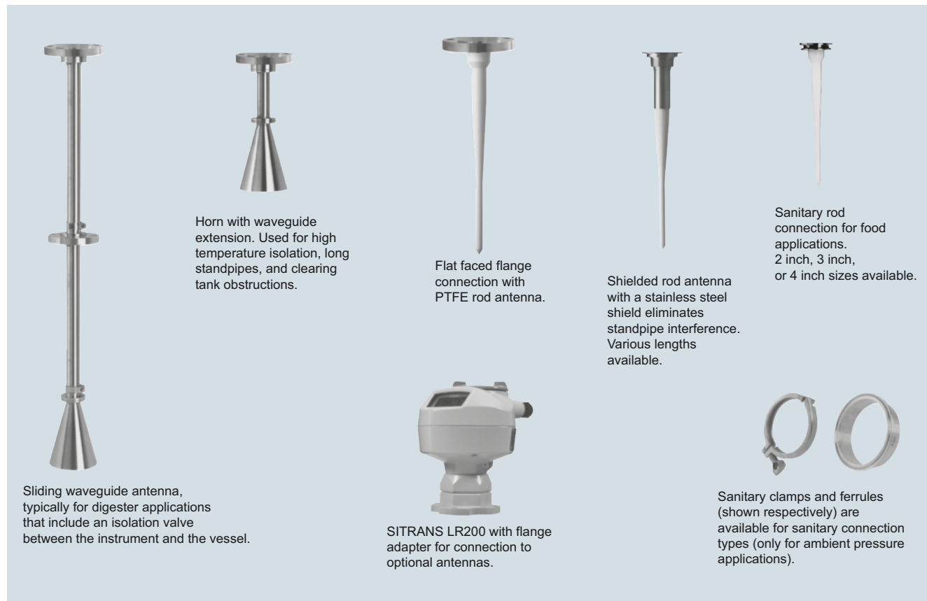
Antenna configurations for SITRANS LR200
