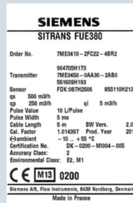
FUE380 transmitter label (with MID first verification)
