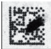
Figure 4-7 Damaged surface of the marking or part
