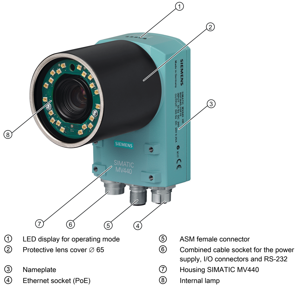
Figure 3-2 Design of the SIMATIC MV440
