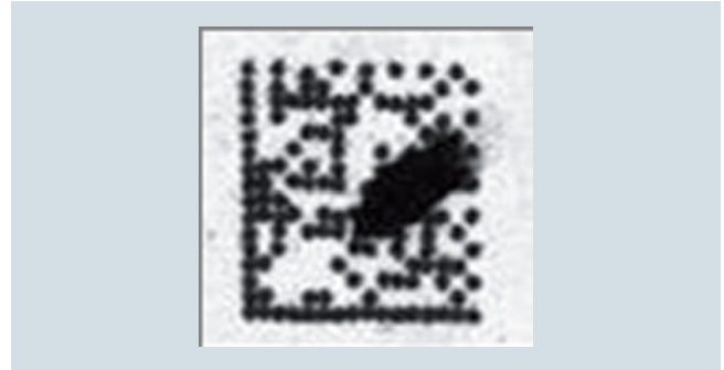
Damaged surface of the marking or part
