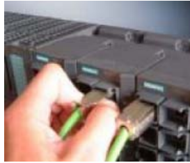
Figure 4-7 Releasing the RJ-45 Plug
