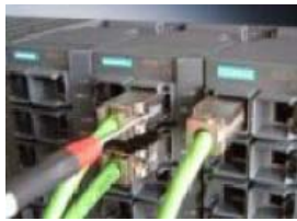
Figure 4-8 Releasing the RJ-45 Plug with a screwdriver
