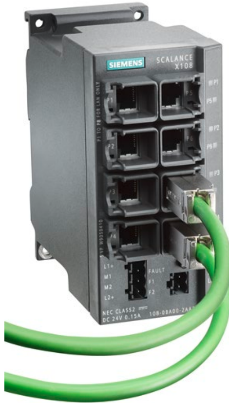
Figure 5-2 Plugging in the IE FC RJ45 Plug 180
