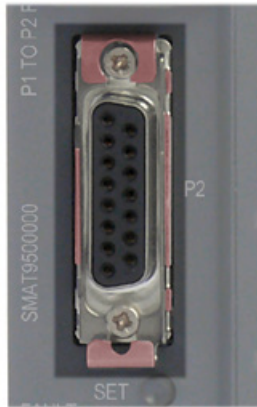
Figure 5-3 Locking mechanism in the open position
