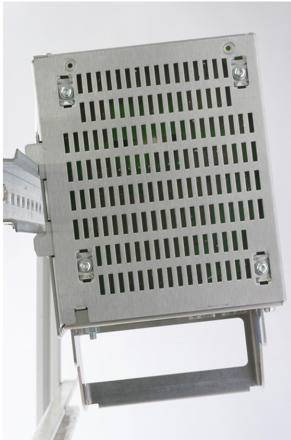
Figure 5-1 Mounting on a 35 mm DIN rail based on the example of a SCALANCE X204RNA EEC
