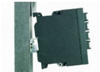
Image 4-2 Removing from a 35 mm DIN rail
