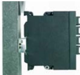
Image 4-1 Mounting an IE Switch X-300 on a DIN rail (35 mm)
