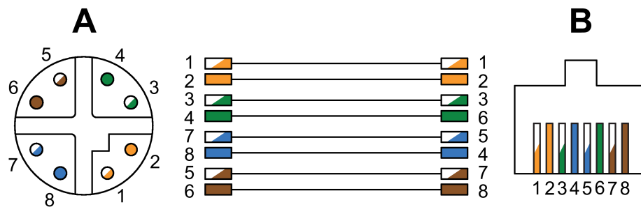
A Front view of M12 connector, X coded according to IEC61076-2-109
