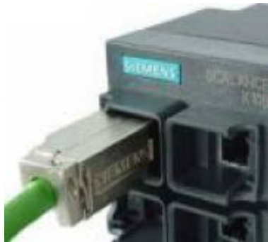
Image A-2 Inserting the IE FC RJ-45 Plug (based on the example of the IE FC RJ-45 Plug 180)
