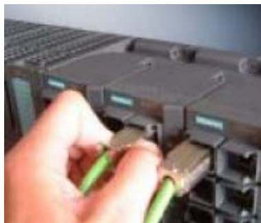
Image A-3 Releasing the RJ-45 plug (based on the example of the IE FC RJ-45 Plug 180)
