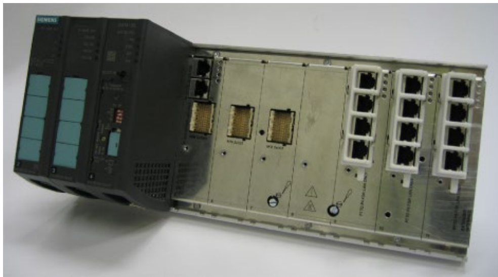
Figure 3-8 Basic device without media modules, protective caps and covers
