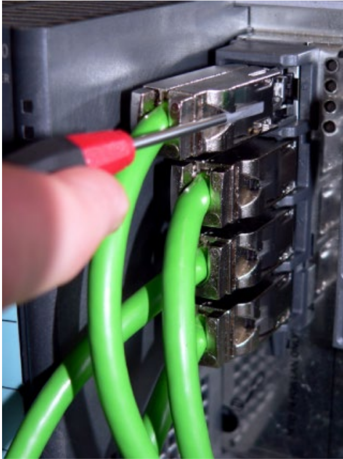
Figure 5-9 Unlocking the FastConnect RJ-45 plug
