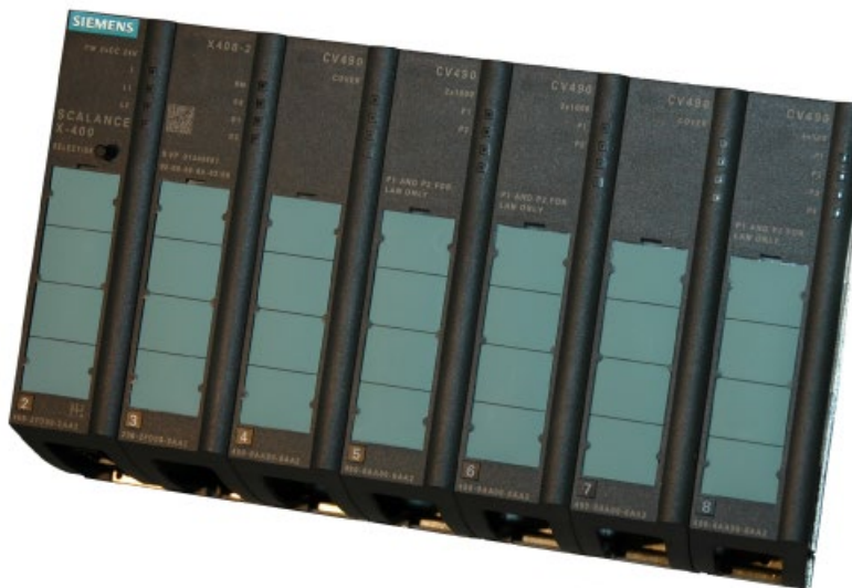
Figure 3-18 SCALANCE X408-2 basic device with media modules and covers
