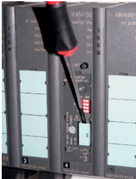
Figure 6-13 Removing the C-PLUG from the SCALANCE X414-3E
