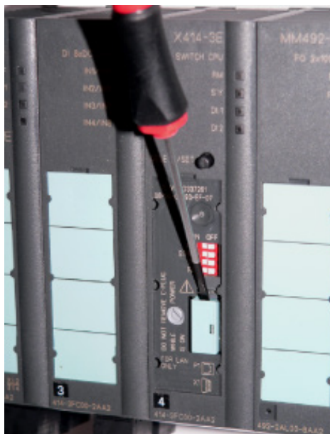
Figure 6-14 Removing the C-PLUG from the SCALANCE X414-3E
