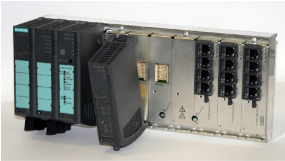
Figure 4-5 Inserting a media module
