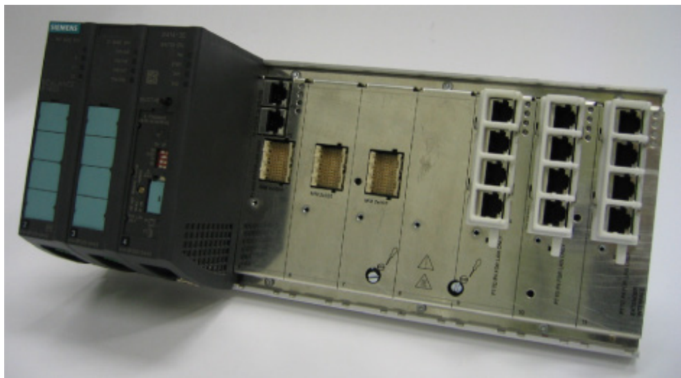
Figure 3-9 Basic device without media modules, protective caps and covers
