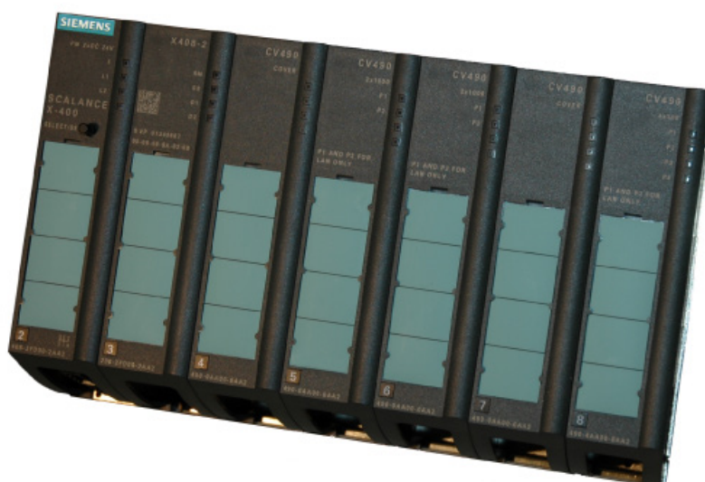
Figure 3-19 SCALANCE X408-2 basic device with media modules and covers
