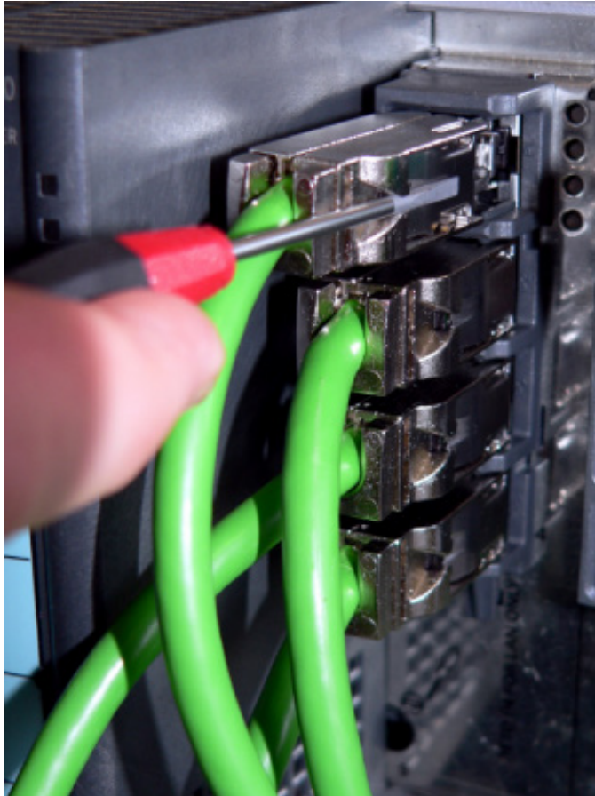
Figure 5-9 Unlocking the FastConnect RJ-45 plug
